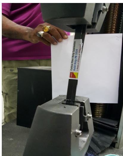
Tensile Strength Testing Equipment, Method of Tester Installation, Once Tested the CFRP Cured Laminates or CFRP Pultrusion Laminates Breaking
