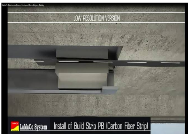
11] Install the Build Strip PB in Position
